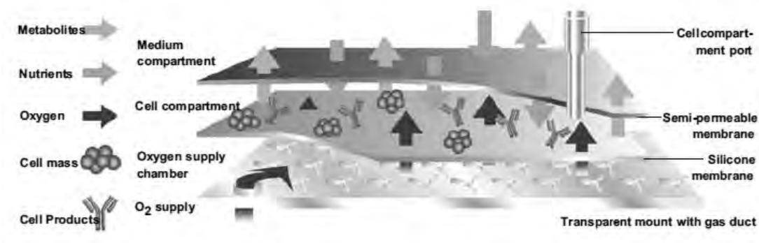
Fig. 1 Schematic View of the CELLLine Two-Compartment Technology
