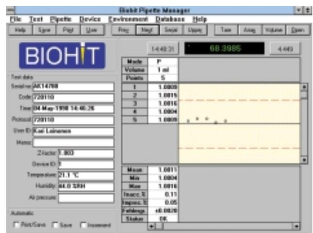
Figure 2. Performance checking of a pipettor using the gravimetric method monitored by a computer.
